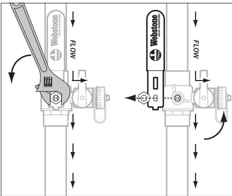
1. Turn handle nut counter clockwise to loosen nut. Remove nut and handle.
