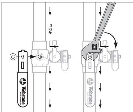
2. Replace handle in desired operating position. Replace and tighten nut.
