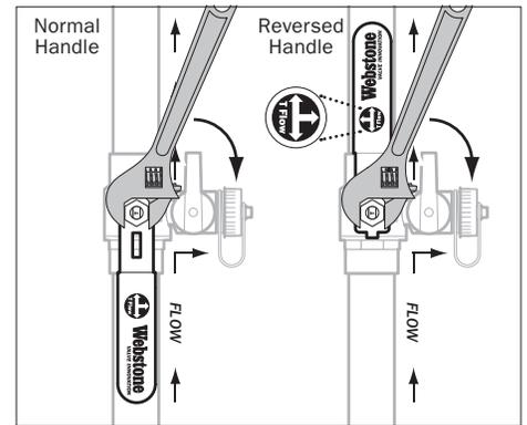
3. Replace handle in normal or reversed position. Replace and tighten nut.
