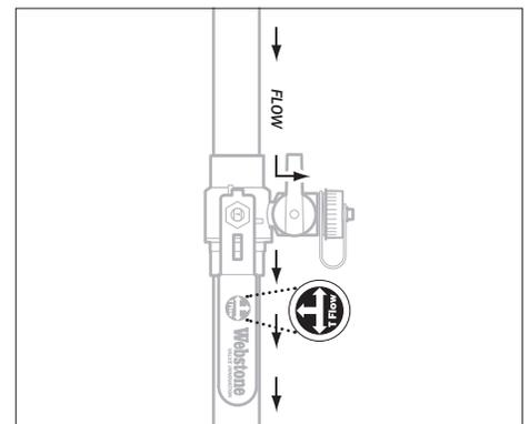
3. If necessary, use enclosed T-Flow sticker to indicate correct flow path on handle. T-Flow logo will match "T" stamped on end of stem.
