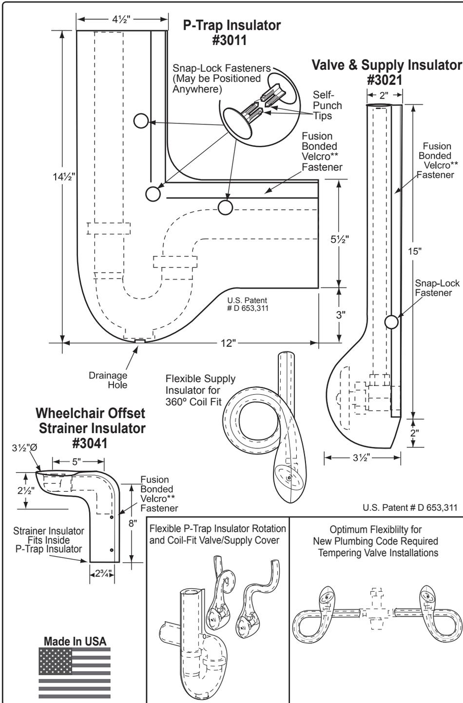
Flexible P-Trap Insulator Rotation and Coil-Fit Valve/Supply Cover
