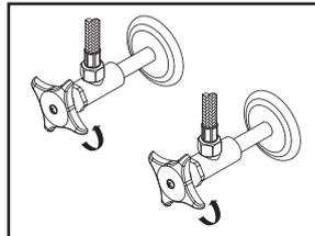
(6) Connect hot and cold inlet supply hoses to supply stops. For 1/2" connection; use 3/8" male to 1/2" female adapter for installation. Adapters are optional and not provided with faucet. Turn on both side supply stops.
