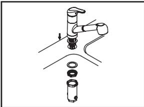
(2) **For 1-Hole Installation:-** Make sure washer is under escutcheon, slide escutcheon for 1-hole installation to the faucet body. Insert faucet through mounting hole. Make sure spout swivel angle are even to the right and to the left. From underneath of the sink, thread locknut and washer to the faucet body, tighten locknut with help of supplied mounting tool.
