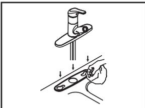
(3) **For 3-Hole Installation:-** Thread mounting bolts to deck plate. Apply plumbers putty under the base gasket. Place faucet with deck plate in position on the sink. Make sure spout swivel angle are even to the right and to the left. From underneath of the sink, thread locknut and washer to the faucet body, tighten locknut with help of supplied mounting tool.
