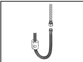
(5) Connect spray head hose to faucet outlet hose from underneath of the sink. Install weight on spray head hose, adjust weight's position so the spray head can be retracted properly.
