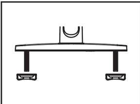
(4) Thread and tighten both mounting nuts to mounting bolt to secure deck plate.
