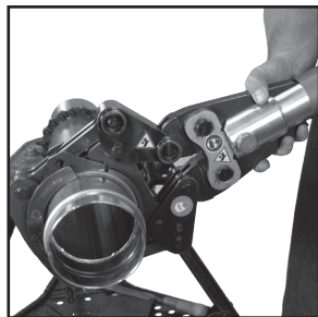
Figure 8: Placement of adapter jaw into pressing chain
