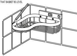
DRILL HOLES: Ø 3/16" [Ø 5mm] IN DRY WALL OR Ø 1/4"[Ø 6mm] IN TILE
