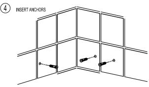
THE BASKET FRAME AND METAL POSTS AND INSERT MOUNTING SCREWS THROUGH
