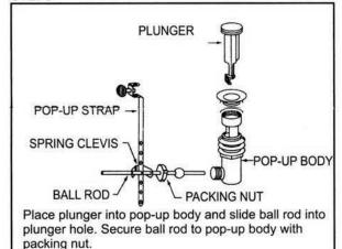
Place pop-up strap and spring clevis over ball rod as shown.
