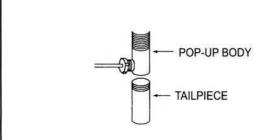
Put pipe compound on tailpiece and thread into pop-up body hand tight.
