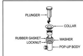
Remove collar and plunger from pop-up body. Turn locknut down as for as it will go and install washer and rubber gasket.
