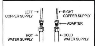
Carefully bend the copper supplies to meet the supply lines. Use the palms of your hands to bend, so as to avoid kinking.
